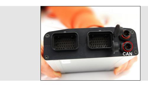
On this connector are both CAN and RS232 Protocol. Here below is the connector pinout as well as the connection table.
