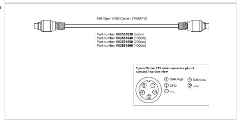
Used to connect the ACC2 Open to the PC and power the sensors. This cable is necessary when you need to check the channels values on the PC through the OnLine feature or you need to calibrate the sensor.
