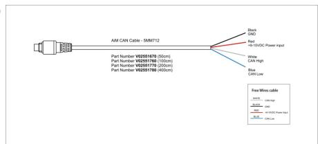
Used for connecting the ACC2 Open to a device through CAN and get the power.
