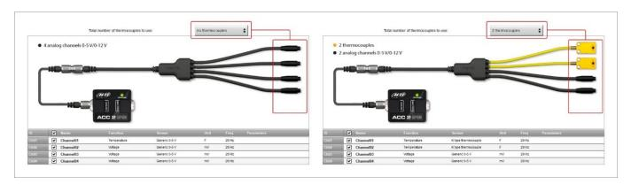
ACC2 Open supports up to four K type thermocouples. Once the number of thermocouple(s) to be connected is fixed the software warns you and the corresponding channel(s) switches to "Temperature".
