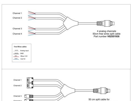
Harness for 2 thermocouples and two AiM sensors.
