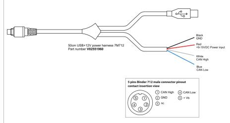
Used for connecting the ACC2 Open to the PC for the configuration. This cable may be used for configuring the ACC2 Open but does not allow you to evaluate the channels OnLine or to calibrate the sensors.
