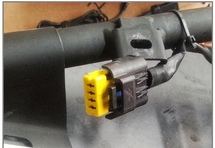
Connect AiM wiring to Ducati wiring as here on the right.
