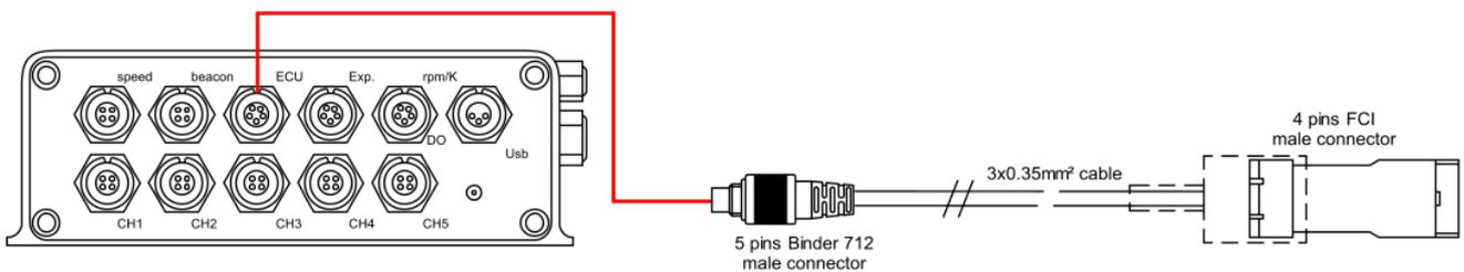
To connect AiM EVO4S to **V02569170** cable use the seven pins Binder 712 female connector labelled "ECU" on the logger front as shown here below.
