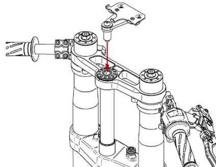
Tighten the M8 screw and the distance piece until the assembled brackets about the bike fork.
