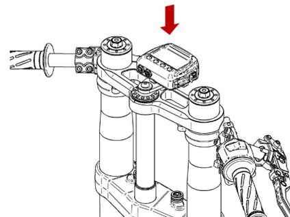
Tighten Solo bracket screws.
