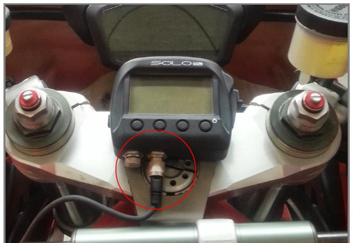
To connect AiM SoloDL to **V02569170** cable use the seven pins Binder 712 female connector placed right under the logger as shown here below.
