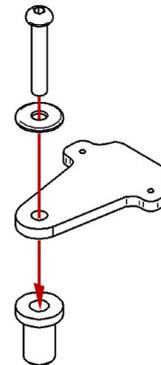
Fix Solo bracket to Panigale one using the two countersunk screws you find in the kit.
