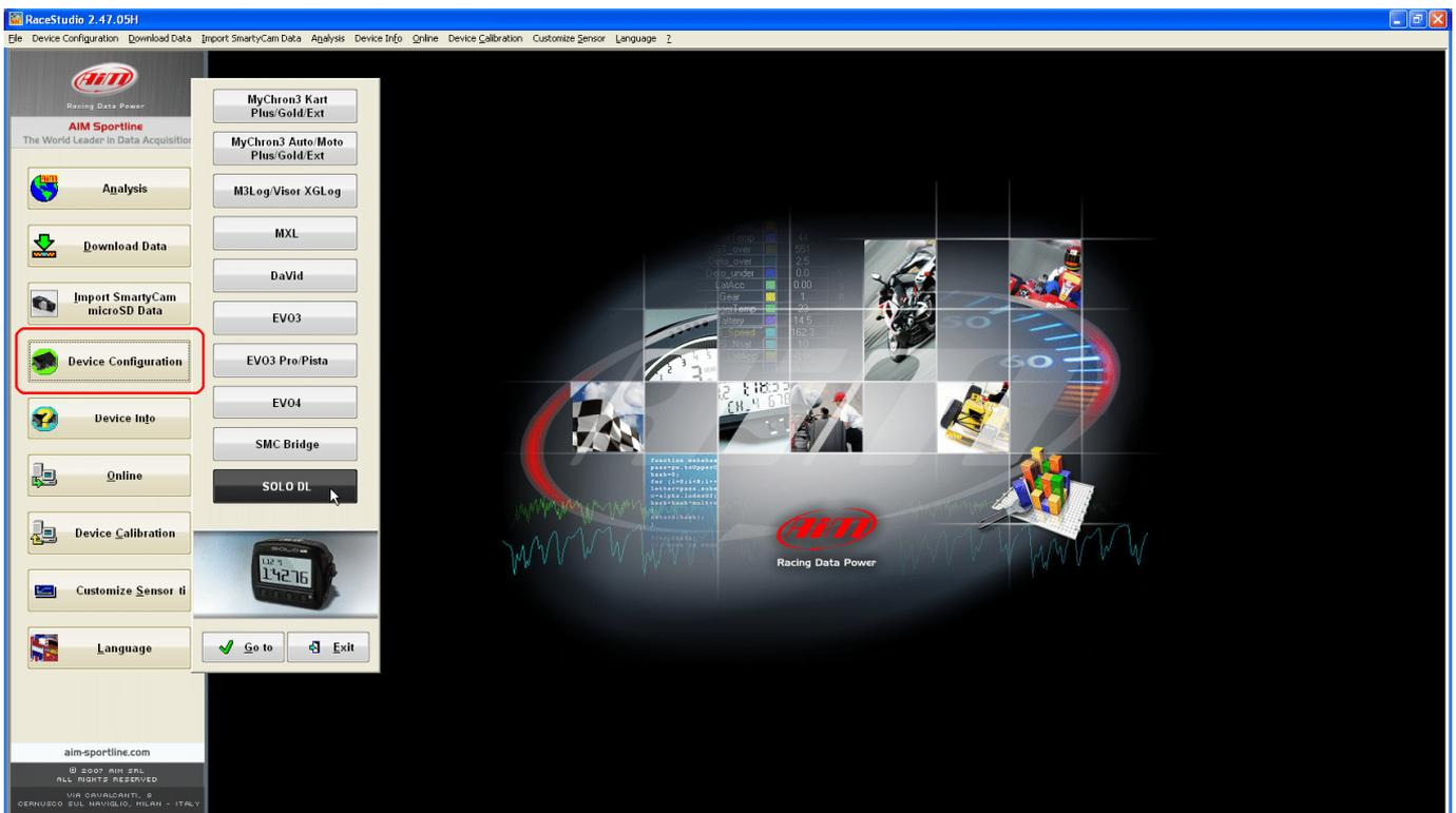
The software shows SoloDL configuration page: press “Configuration Manager” and select the configuration you want to use or press “New” to create a new one. In this second case “New configuration” panel appears: select ECU Manufacturer “Microtec” and ECU Model “M222” as here below.
