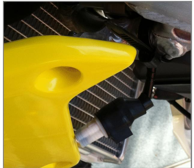
Remove the black rubber cap sliding it along the cable as shown here on the right.
