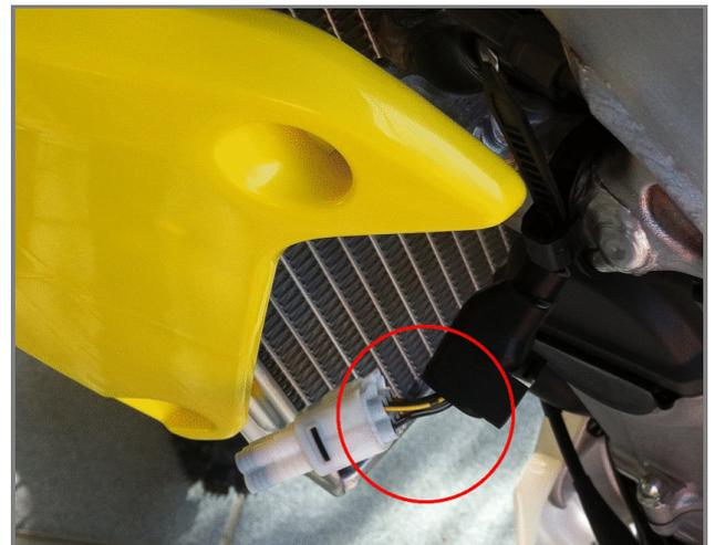
Unplug Suzuki cable as shown here below and in the image.
