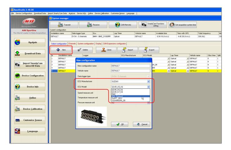
Confirm pressing "OK" and transmit the configuration to EVO4 pressing "Transmit".
