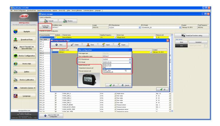
Confirm pressing "OK" in both panels and transmit the configuration to SoloDL pressing "Transmit" as shown below.
