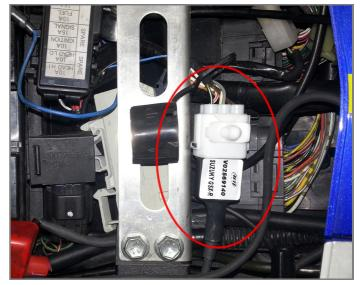
If you have installed an AiM **EVO4** logger take the cable to the logger.
