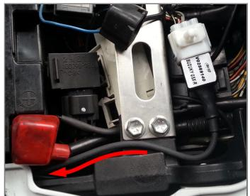
Make the cable pass between the fuel tank and the chassis as in the image on the right.
