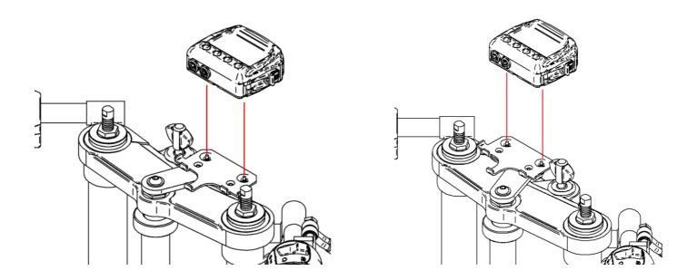
Fix it using the screws already inserted rear on Solo/SoloDL bracket.
