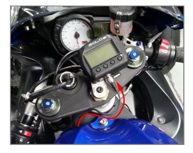
To connect SoloDL to male Binder connector of **V02569140** use the female Binder connector placed bottom right of the logger as shown here below.
