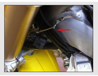
Make AiM cable pass around the fork plate ("F" here below on the left) and connect AiM cable to SoloDL (image on the right).
