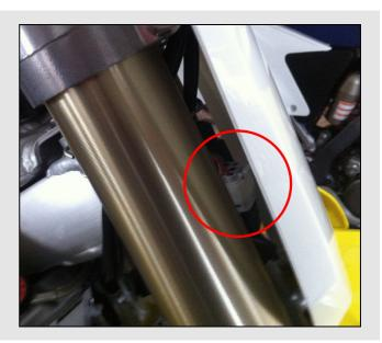
The connection is to be made as explained in the previous paragraph. Once this operation performed, the cable you connected has to pass between the bike plate and the bar pad. Images here below show the cable path.
