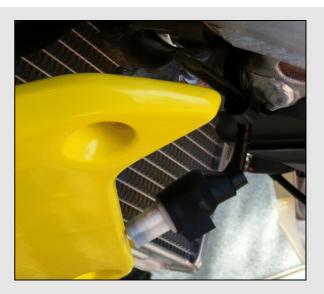
Remove the black rubber cap sliding it along the cable as shown here on the right.
