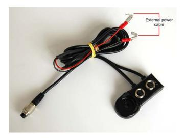
Four ways **Data Hub**, on the contrary, need the proper optional cable for external power to be plugged in one of the 4 inputs.
