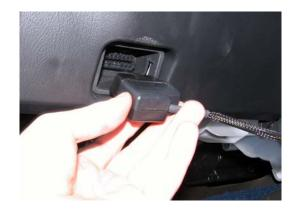
It is possible that all parameters managed by the ECU are sent on the OBDII plug. Refer to paragraph 3.1 for further information concerning the channels that can be shown on **SmartyCam** videos.
