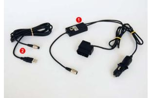
**ECU Bridge CAN/Kline kit** : **ECU Bridge** with OBDII connector, allows to remote the connection on the vehicle OBDII plug. The kit includes:
