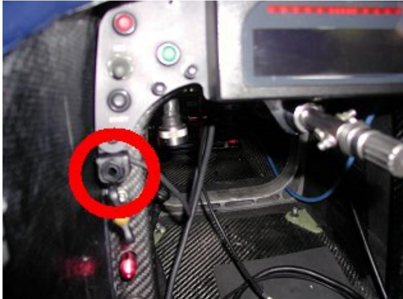
It is suggested to install the USB female connector (used to configure the system and to download data) in the body cell, under the display, as shown above.
