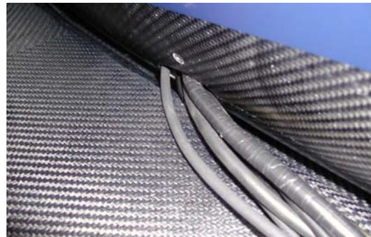
Once reached the vehicle body, it is suggested to use the proper cable passage situated near to the battery on the left side of the vehicle, as shown in the figure below.
