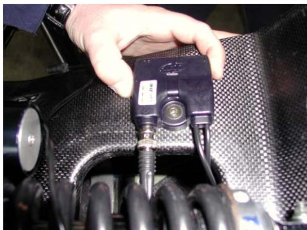
**GPS 03 Module** communicates with **EVO3 Pro** using CAN bus CAN 0.
