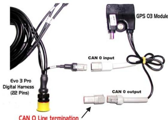
It is strongly recommended to verify that CAN termination connector is correctly plugged in: then connect DTM connector to the **EVO3 Pro** digital harness (22 pins) as shown in the figure above.
