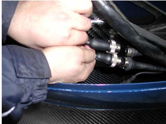
The connection to CAN bus CAN 1, that allows the communication with Magneti Marelli MF4-L ECU, is made through J59 connector of **EVO3 Pro** digital harness, placed in the left side of the vehicle body. J60 connector, on the other side, sends the “end lap” signal to the vehicle dashboard.
