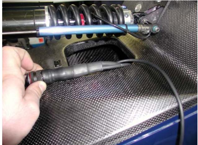
Use plastic wrappers to fix the digital (22 pins) harness to the other cables of the engine plant.
