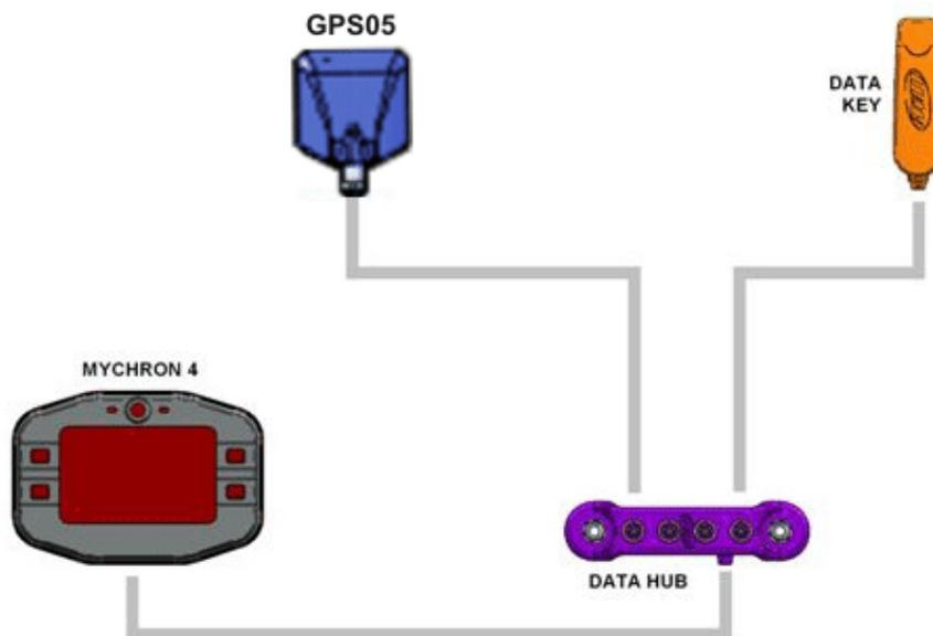
The figure above shows a CAN network powered by **MyChron4** internal batteries: this powering reduces network autonomy, valuable in around two hours recording time.
