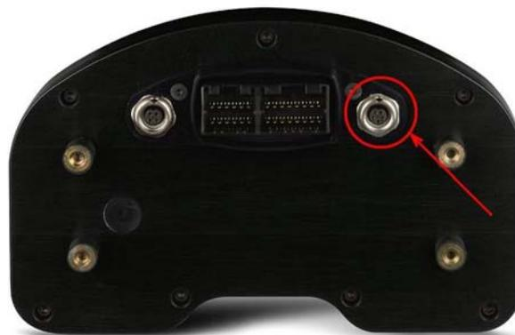
To connect **MXL Pro** connect **GPS05 Module** to the CAN cable labelled EXP (expansion) of the logger wiring.
