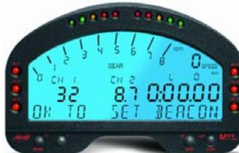
Once start/finish line is set, if the system is configured to capture splits, the page shown below appears; reach the point of the track to be considered as split and press “OK” button.
