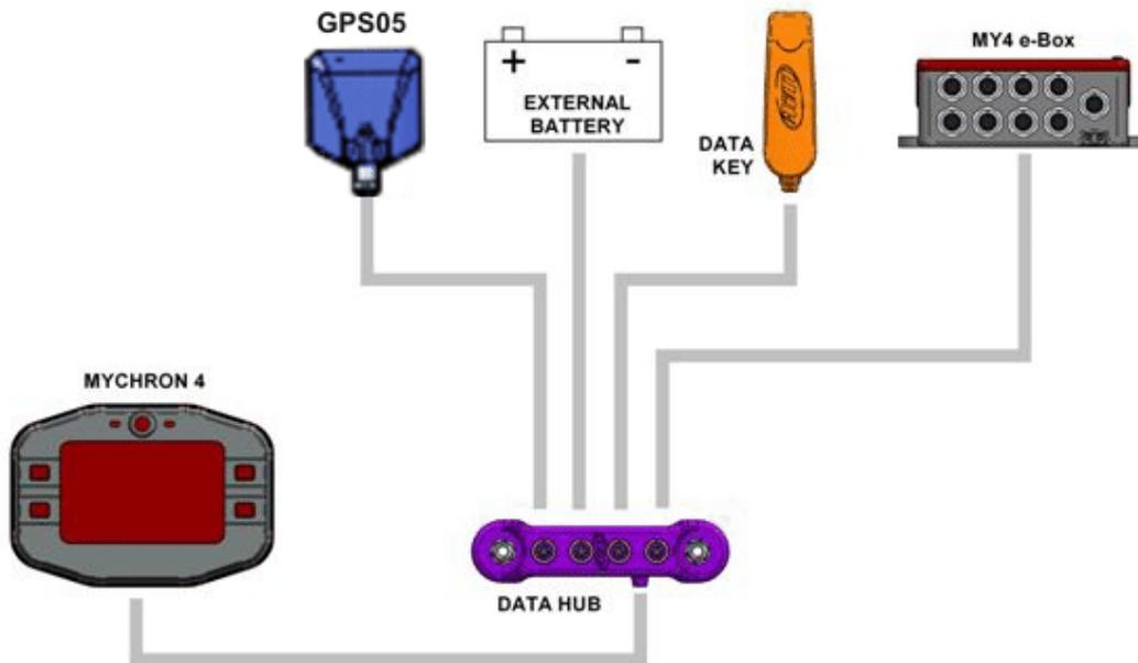
The all network is externally powered. It is recommended to leave **MyChron4** and **eBox** internal batteries at their place.
