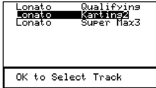
Use MENU/>> and “<</OFF” buttons to scroll the list and “MEM/OK” button to select a track. The system informs that the track has been selected with the symbol “▶▶” as shown here below.
