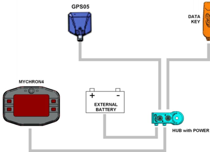
The figure below shows a CAN network where **GPS05 Module** and **MyChron4** are externally powered (assuming a 12 volts battery is available on TAG kart).
