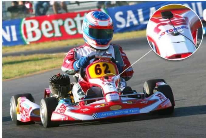
The number plate is made in plastic and the magnet cannot keep the module steady. For the optimum installation we would suggest to use a strip of Dual Lock – Velcro®. The **GPS05 Module** cable should pass on the kart front fairing as shown below.
