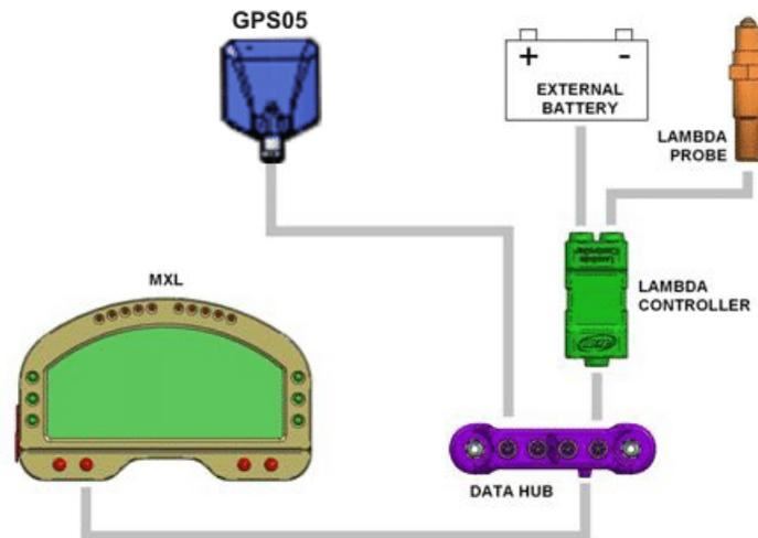
The figure above shows a CAN network of **LCU-ONE** and **GPS05 Module**. Peripherals can be connected to **Data Hub** using one of the 4 CAN inputs. The CAN network can be further increased using the same logic.
