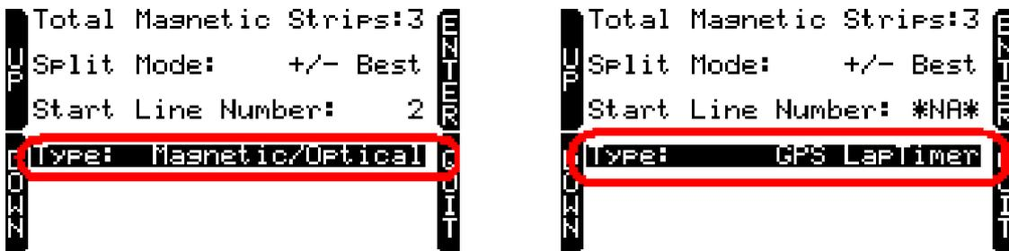
Selecting “GPS Laptimer” it is possible to leave the optical/magnetic receiver connected and the system will automatically disable it when **GPS05 Module** with lap timer function is connected.
