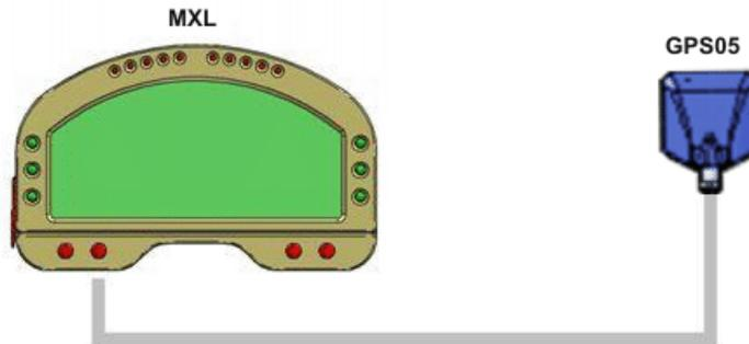
The figure above shows a CAN network made of **MXL Pista** and **GPS05 Module**. To connect **MXL Pista** to **GPS05 Module** use the 5 pins connector mounted on the logger back side as shown below.
