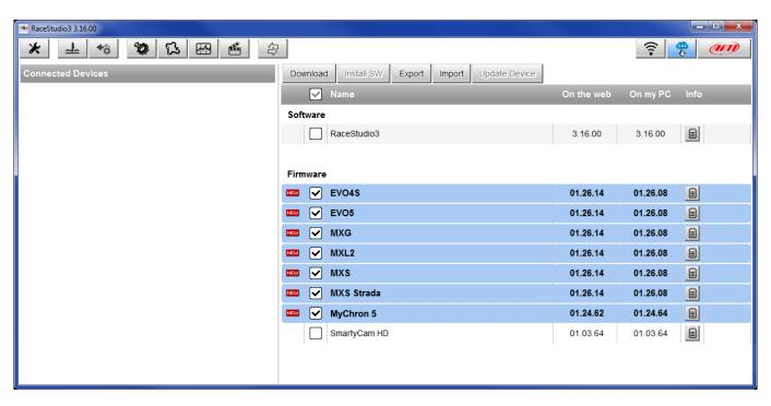
Once the new firmware has been downloaded connect your device to the PC using the USB cable included in the kit to perform a firmware upgrade. In a few seconds the device is ready.
