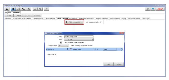
The Status variables can be used as any other channel, so they may be seen online, transmitted to the CAN stream, recorded, used for triggering a command or for turning ON a LED or an Icon.
