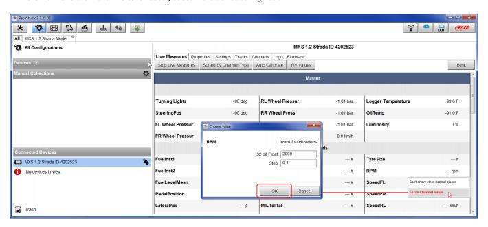
As shown in the image below, once the values have been forced they are shown right of the page hedged in red. With the two "+" and "-" lateral buttons it is possible to change the forced values.
