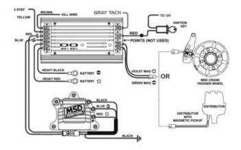
The output labelled "GRAY TACH" gives a 5-50V output that can be directly sampled by MX Strada series dash.
