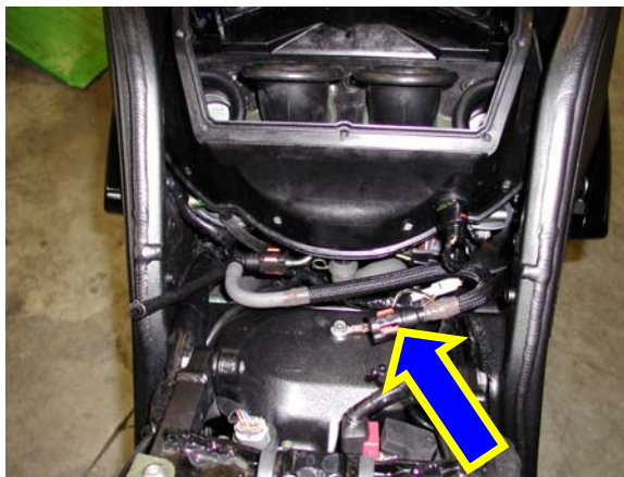
Figure 18: the hose that takes the fuel to the engine
