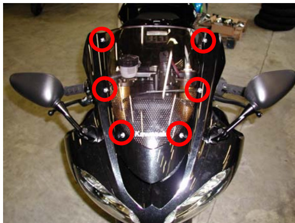
Figure 1: front transparent fairing – screws location
