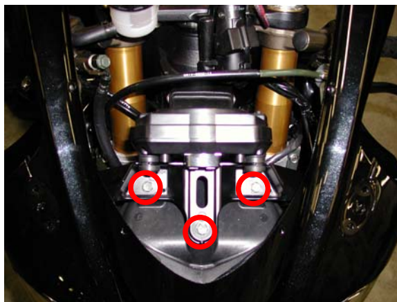
Figure 5: the screws that fix the stock dash to an internal chassis
