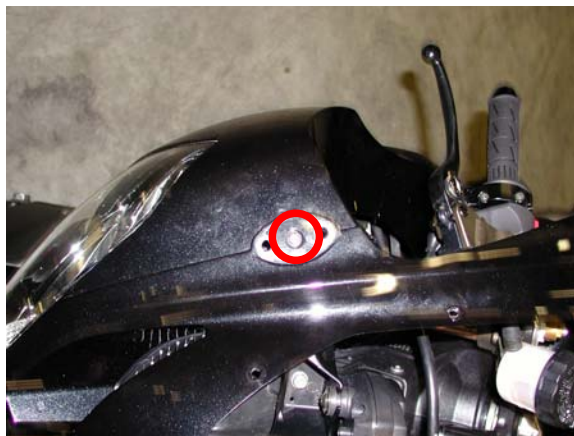
Figure 3: central external screw.
