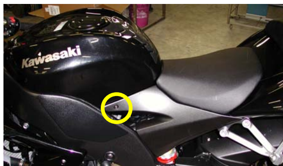
Figure 14: the screw that fixes the plastic fairing to the bike chassis
