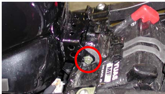
Figure 15: one of the screws that fix the gas tank.
