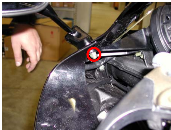
Figure 2: .internal screw to remove.
