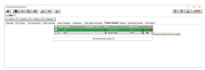
The setting panel appears: fill it in. In the example Power output 1 has been configured to manage a fan: it turns ON when Water temperature is greater than 90°C: Max accepted current (Maximum value of requested Loan) is 8 Amp: over this value the output circuit opens and the read status becomes "Overcurrent".
