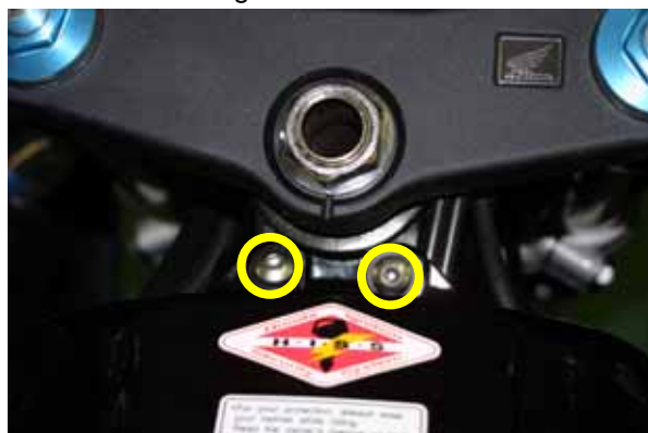
Figure 4: The two front screws of the gas tank.
