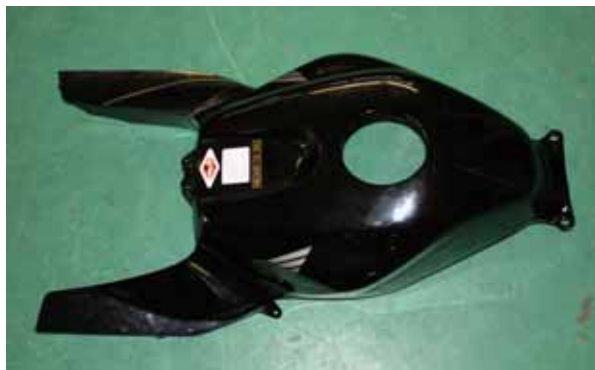
Figure 13: the gas tank fairing has been removed.
