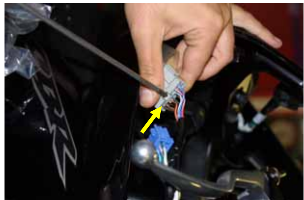
Figure 17: unplugging the on-board connectors
