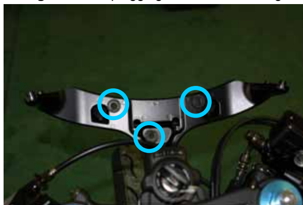
Figure 20: holes of the anchor plugs of the on board dash
