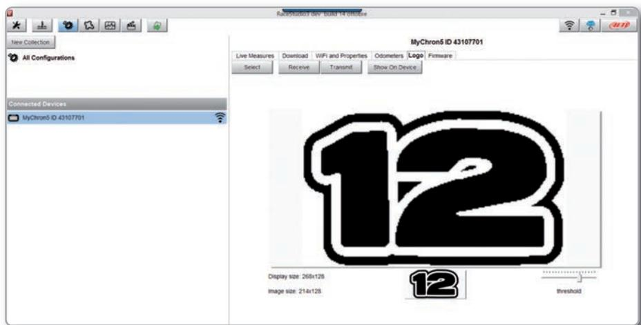
You can easily select a picture (JPEG or BMP) in your PC and transmit it to ( or receive from) the MyChron5
