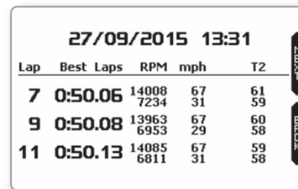
It shows the best three laps of your test, giving the information about maximum and minimum RPM, speed, and temperature(s) for them.
