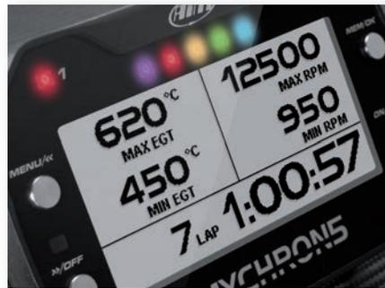
There are two RGB alarm LEDs: you can configure the color, blinking frequency and event to which to connect them.
