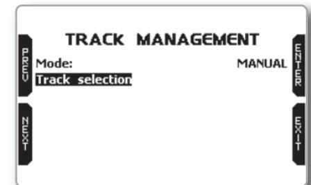
■ **Manual:** Allows you to select the desired track from the internal database. The manual mode is to be preferred when there are different track configurations nearby.
