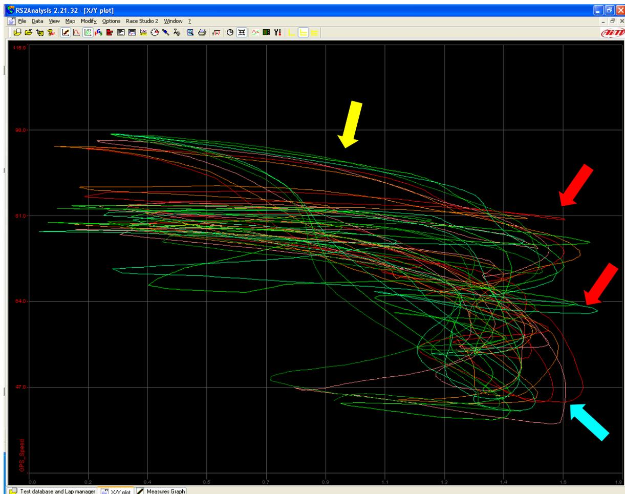
In the second part of the track we can see how Morbidelli better advantages of grip at very high speed (yellow arrow in the figure, Morbidelli's red lines are more rightwards). The Casaccia hard braking is the last point where Morbidelli gains on Dovizioso, better managing the first part of the hard braking.
