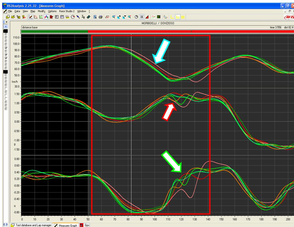
On the main straight slip value is 1 and goes under 1 during brake.
