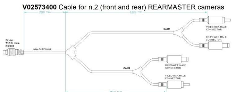
\* The two **DC Power** and **Video RCA** cables couples are respectively 4m and 6m long, in order to allow both front camera and rear camera connection.
