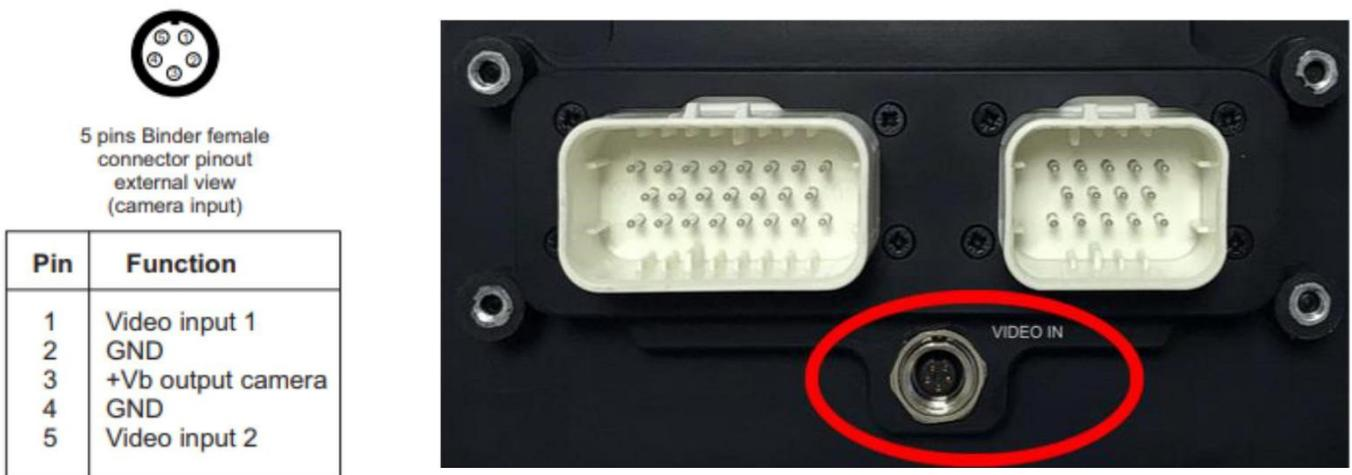
The Video In connector allows the connection of two different Rear cameras, that may be activated as here down described.
