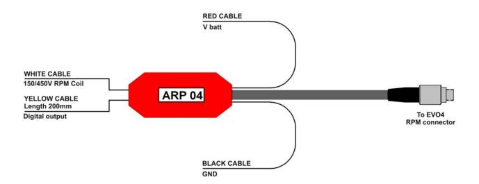
It can happen that RPM signal, sampled from the coil, is not correctly sampled by **EVO4**: it can be very instable or the value shown does not correspond to the real one. This problem can depend on electrical interferences that causes noise peaks. RPM coil adapter filters the signal. The images here below show an RPM signal out coming from the coil on the left and the same signal filtered on the right.
