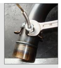
**Warning:** when running the thermocouple cable along the chassis keep it as far as possible from other cables (like RPM cable or receiver one) to minimize possible interferences.
