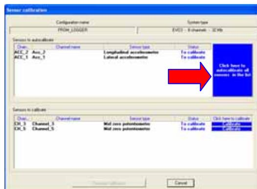
Press “Click here to auto-calibrate all sensors of the list” button (highlighted with a red / blue arrow in the above figure): the software auto-calibrates automatically all channels of the “to be auto-calibrated” box.
