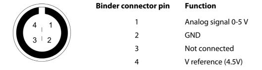
The kart steering potentiometer **electrical characteristics** are:
