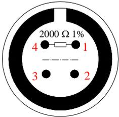
**4 pins Binder 719 male connector solder termination view**
