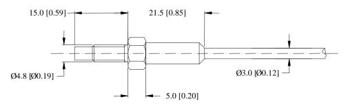
M5 thermo resistor – **Dimensions** in millimetres [inches]
