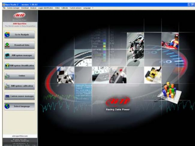
To make the system recognize the sensor it is required to **create a custom sensor**. Press “Custom sensor manager” on the left vertical keyboard or on the menu bar of the software main window. “Customize Sensor” window, shown on the right, appears.
