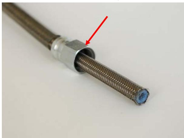
Insert the nipple under the metallic braid as shown here on the right, pressing it until the contact with the internal part of the pipe (labelled as "A" in the figure below) is complete and covering it with the metallic braid.
