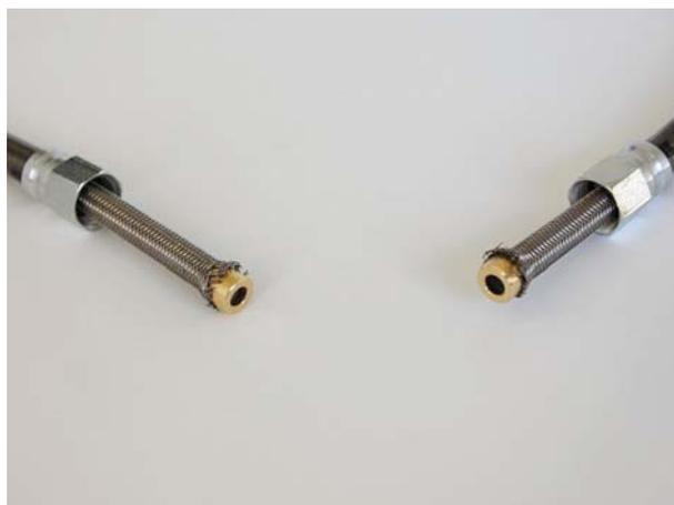
Establish the exact junction position - as it will determine the sensor position - before tightening (making a reference mark).
