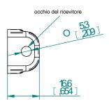
Optical receiver - Dimensions in millimetres [inches]
