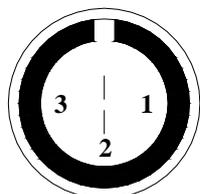
3 pins male Binder 712 connectors pinout: solder termination view
