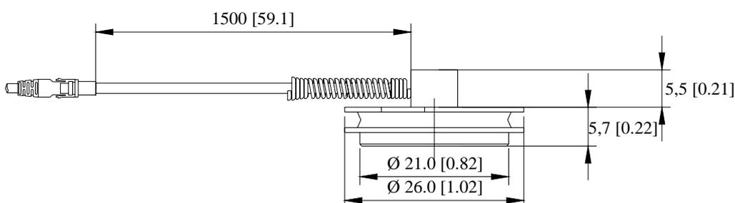
Thermoresistor CHT (front view) - Dimensions in millimetres [inches]
