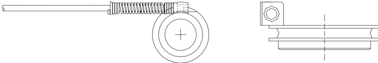
**Figure 1:** Cylinder head Thermoresistor (top and side view)
