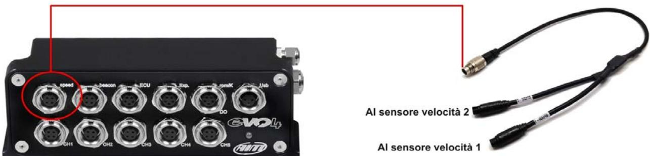
Here below is the cable constructive scheme.
