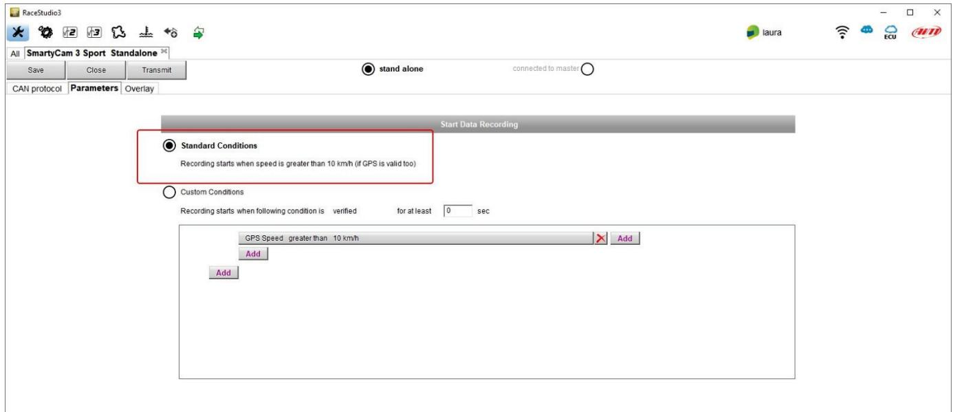
If SmartyCam 3 is **connected to a Master** it starts recording when the master does.
