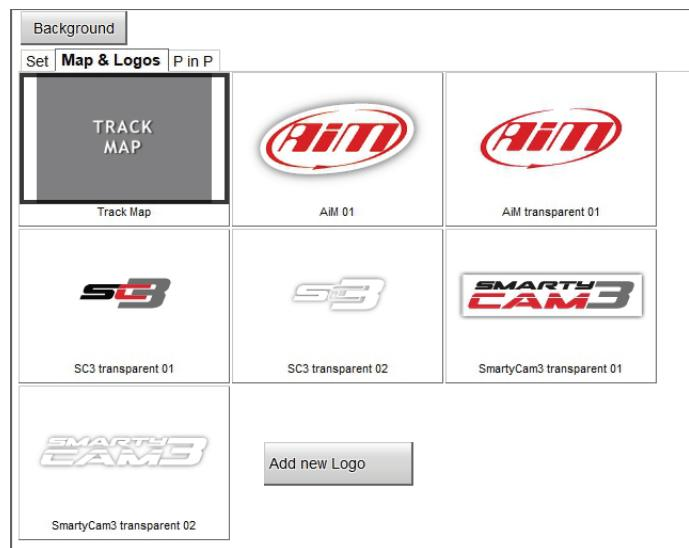
Please, note that, when configuring SmartyCam 3, you only set position and dimension of the track map while the shape of the circuit dynamically changes according to the circuit you are racing on.
