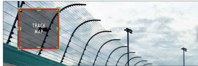
Here on the right you see an overlay where both track map and secondary camera as Picture in picture (**SmartyCam 3 dual only**) are set.
