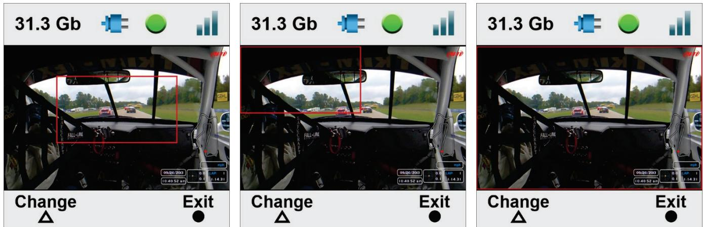
**SmartyCam 3 Dual** has two bullet cameras: you may select the one for which you like to set the exposure.
