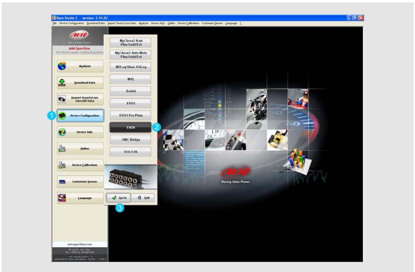
Select the configuration where the calculation is to be set or create a new one.
