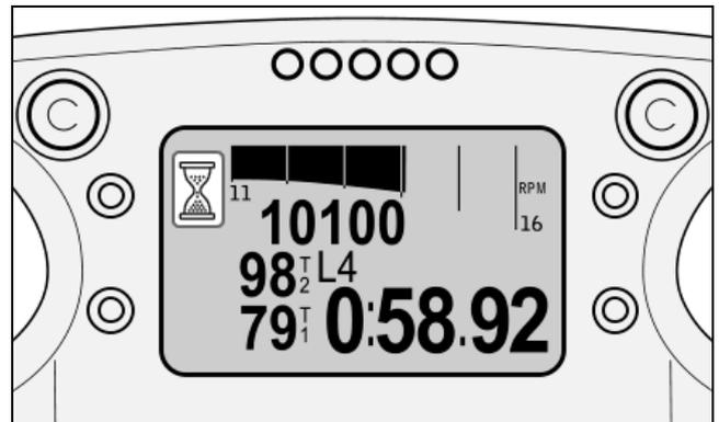
If EVO4 is connected to a MyChron3 Dash, the gear display will be empty till when the gear is not properly calculated.
