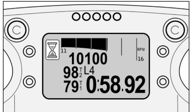
If ECU Bridge is connected to a MyChron3 Dash it will show the gear display empty.
