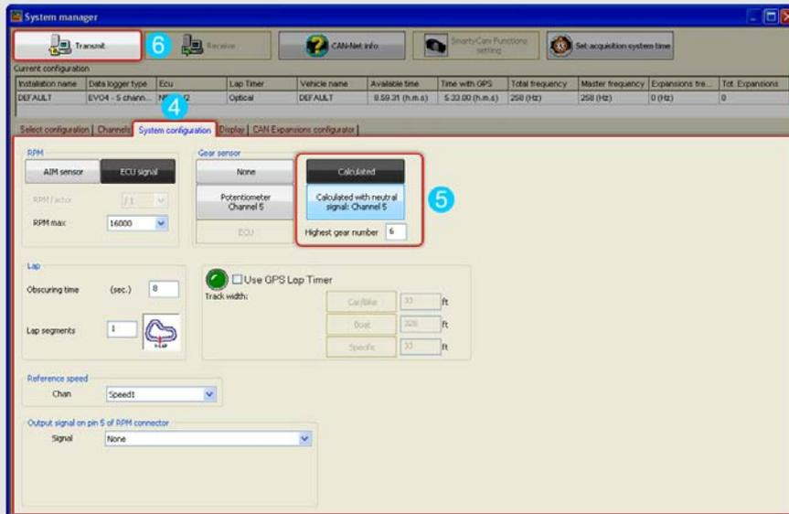
If EVO4 is connected to a Formula steering wheel, when powered on – before starting the calculation – it will show a hourglass where the gear is set to be shown.
