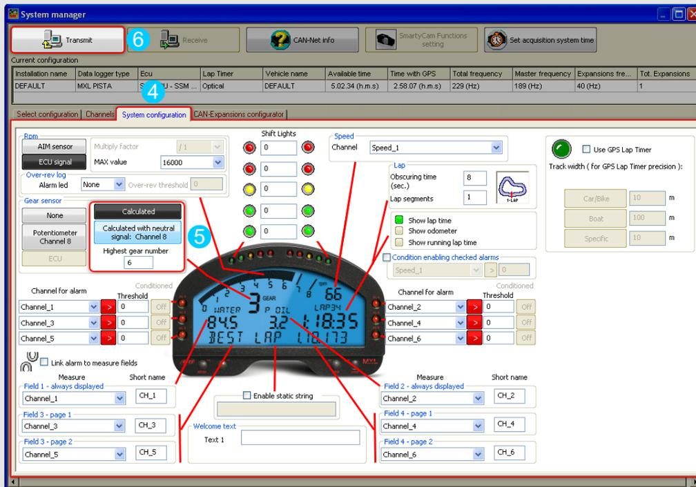
Then enter "System configuration" layer (4), set "Calculated" (5) – motorbikes can opt for "Calculated + Neutral signal: Channel 8" and fill in the highest gear number. Transmit the configuration to MXL (6). At power on, before starting the calculation MXL display shows "running gear cal".
