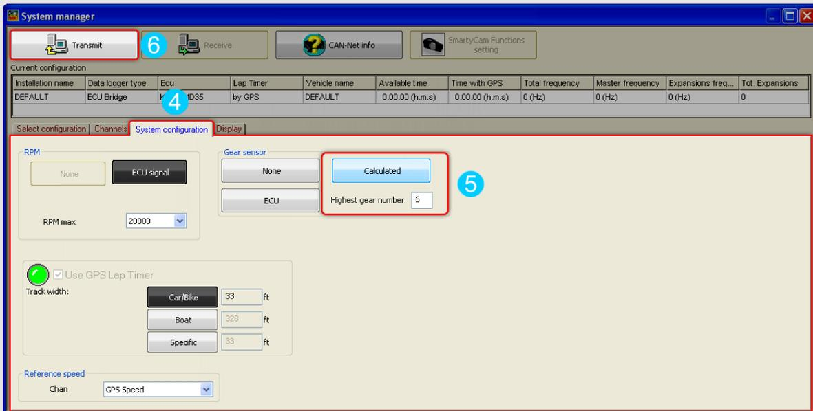
Go to "System Configuration" layer (4), set "Calculated" gear and fill in the highest gear number. Transmit the configuration to ECU Bridge (6).
