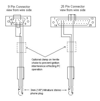
Connection between DB9 Autronic cable and AIM loggers is provided by the following pins:
