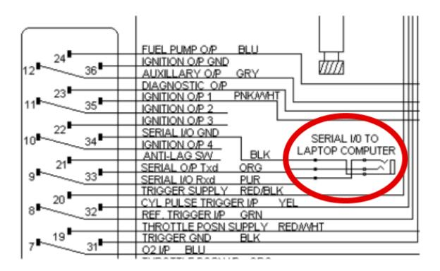
Here below you see the Autronic PC Serial data link spiral cable – to connect DB9 male connector to the Serial I/O and related pinout.
