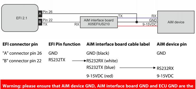
same and do not use pin 15 of EFI ECU "B" connector for GND signal.
