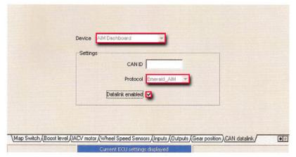
From the "Device" drop down menu select "AIM dashboard". To enable this K3 to AIM data-link ensure the "data link" check box is ticked.
