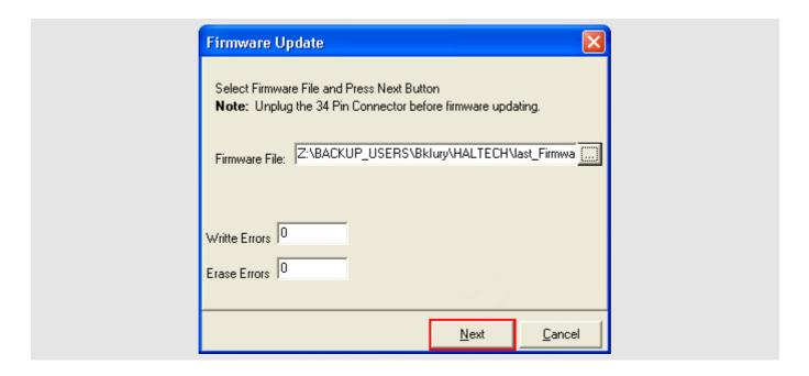
A sequence of four panels appears. Wait, as indicated by the same panels, until the last one says "Updating Firmware Finished press OK" and press "OK" as shown here below.
