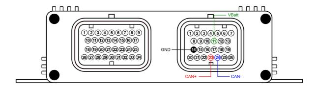
When the firmware has been updated – see chapter 1 – the ECU communicates through the CAN bus on the 26 pins connector. This ECU needs GND and Vbatt connection too. Please refer to your AIM device pinout to connect them. ECU connectors pinout and connection table are shown below.
