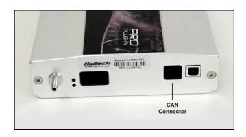
This ECU needs GND and Vbatt connection too. Please refer to your AIM device pinout to connect them. ECU CAN connector pinout and connection table are shown below.
