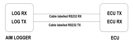
Link G4 ECU data transmission is 57600 Baud: for this reason it is necessary to use "Vi-PEC AIM ADAPTOR", which converts and re-transmits data at 19200 baud.
