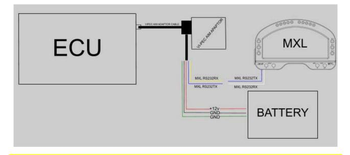
Note: in order to correctly communicate with AIM loggers it is necessary to connect both devices to Vi-PEC-AIM adaptor, supplied with the ECU, that takes bit rate to 19200 bps.
