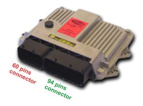
The connector used to connect Magneti Marelli SRA-EDL8 ECU to AIM logger is the 94 pins one.
