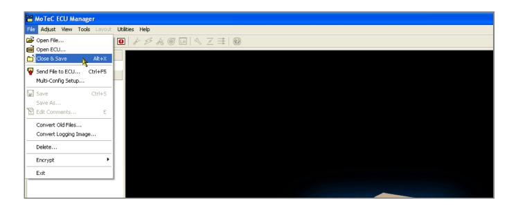
Transmit the configuration to the ECU following this path:
