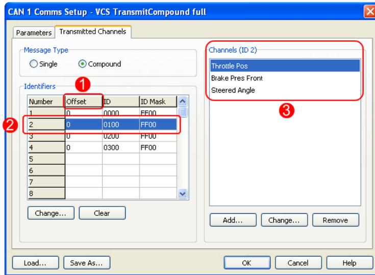
Select the desired channel in the right panel – Channels (ID<sup>2</sup>) – and press “Change” to check the channel settings. Here below are shown the correct settings for Channels (ID<sup>2</sup>).
