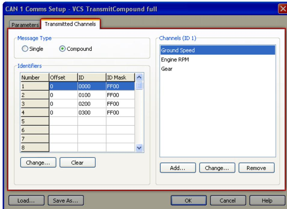
This check is to be performed this way: with an identifier of “Identifiers” panel selected (1) click on a channel of “Channels (ID 1)” panel – in the image here below “Ground speed” (2) – and click “Change” (3).
