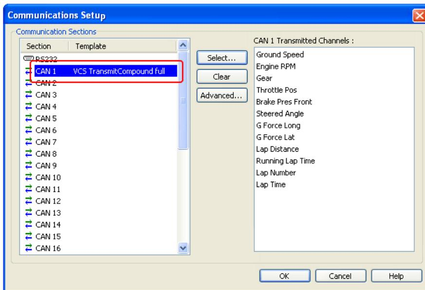
CAN Communication Setup panel shows up: check all parameters and select the CAN line you are using.
