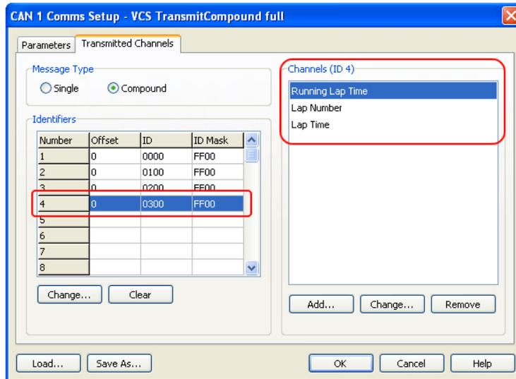
Select each channel and press “Change” to see the related channel setting. Here below are the correct settings for each channel.
