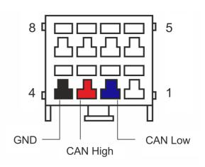
All AiM devices are provided with a 120 Ohm CAN termination resistor. To make them communicate with Nemesis 2 ECU it is necessary to remove it. SoloDL and EVO4 resistor is on the ECU connection cable and it is thereby possible to remove it, while in all MXL the resistor is integrated and it is not removable. For this reason the wiring connection is different. Here below are AMP connector pinout as well as the different connection tables.
