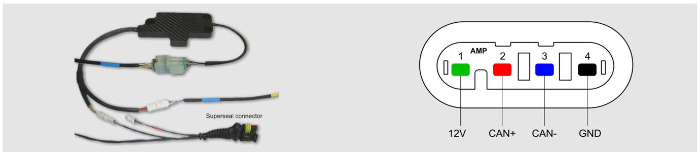
All AiM devices are provided with a 120 Ohm CAN termination resistor. To make them communicate with Nemesis TCS kit it is necessary to remove it. SoloDL and EVO4 resistor is on the ECU connection cable and it is thereby possible to remove it, while in all MXL the resistor is integrated and not removable. For this reason the wiring connection is different.
