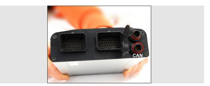
On this connector are both CAN and RS232 Protocol. Here below is the connector pinout as well as the connection table.
