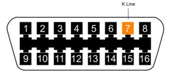
**OBDII connector pinPin functionAiM cable**7K LineK line
