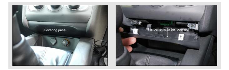
Here the cover has been removed and OBDII plug is shown.
