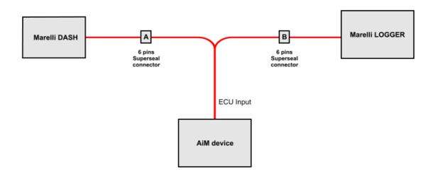
Split apart the two 6 pins Superseal connectors and place AiM device between the two connectors; then follow the table below. Pins number are printed on the connector.
