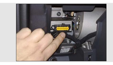
OBDII connector as well as connection table are shown below.
