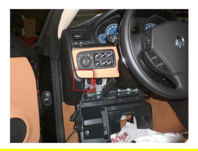
Note: The image above refers to Maserati GT; DLC position can be different on the other compatible cars models.
