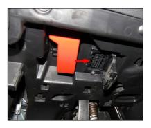
The ECU communicates using the CAN Bus on the OBDII connector. Connector pinout as well as connection table are shown here below
